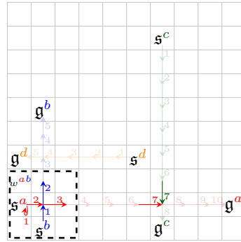
(b) Collision between a and b is repaired by jointly planning inside w^{ab} . The repair creates a collision between a and c at t = 7 .
