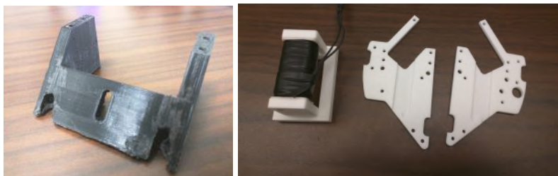
(a) Dribbler Backstop (b) New Kicker Solenoid and Mid Plates
